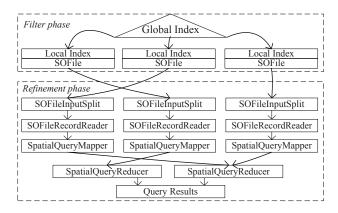
Figure 7. Spatial query processing architecture of *VegaGiStore*. The filter phase searches the global index and outputs candidate SOFile sets; then these candidate sets are processed in parallel by a map-reduce job at the refinement phase.
